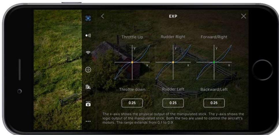
EXP values reflect the logical relationship between the control stick movements you make and the feedback from the aircraft. The X-axis represents how much the control stick is
