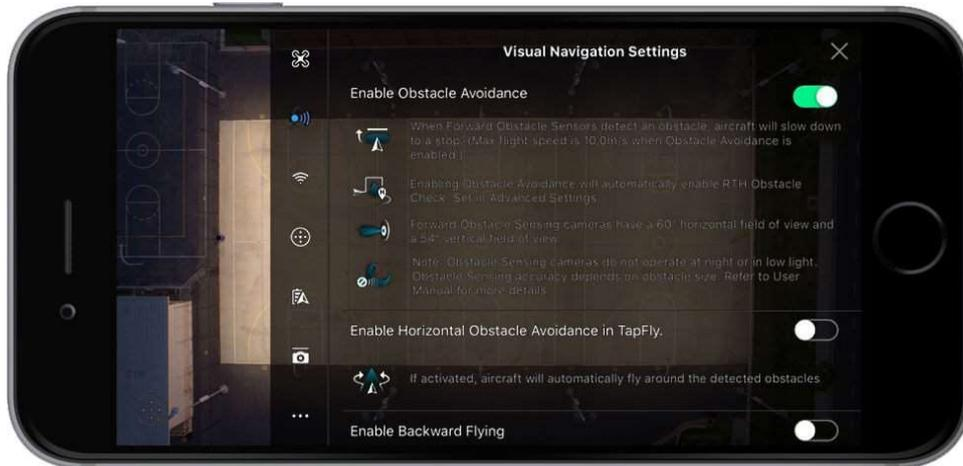
This is where you can control which sensors are on. It is recommended that all the sensors are kept on at all times.
