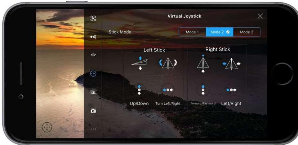
This is where you can choose the stick mode for how to fly your aircraft; the default joystick mode is 2 for both the remote controller and the virtual joysticks. At present, only the Mavic and Spark supports virtual joysticks.
