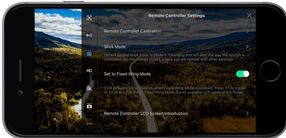
**Remote Controller Calibration:** Here you can calibrate your remote controller's sticks and toggle wheels. You can only calibrate the RC when the aircraft is turned off. To calibrate just follow the onscreen instructions.
