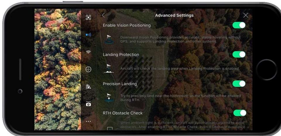
**Enabled Vision Positioning:** If this is toggled then the downwards sensors will be turned on which will help to keep the aircraft in a fixed position when hovering. When turned off your aircraft will drift when it hovers if the GPS signal is too weak.
