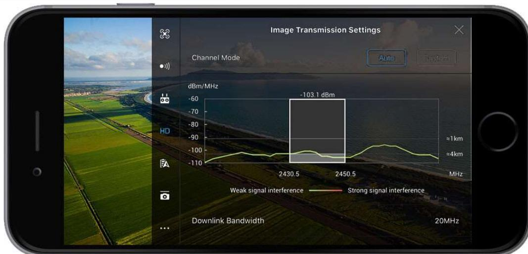
This controls the signal between the aircraft and the remote controller. The signal can be set to Auto or Manual. You can also choose transmission mode for streaming to your mobile device.
