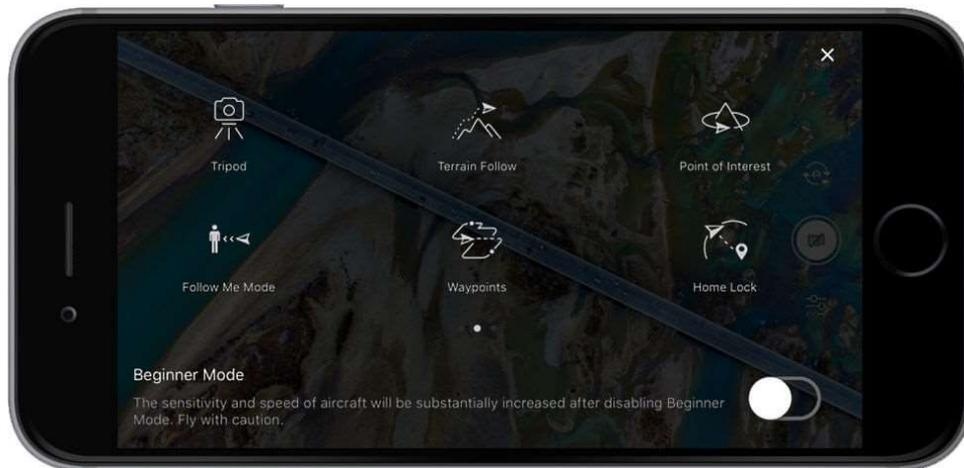
**Tripod Mode:** In Tripod Mode, the maximum flight speed is limited to 2.2 mph (3.6 kph). Responsiveness to stick movements is also reduced for smoother more controlled movements. This mode can only be used when lighting conditions are good, and the drone has a strong GPS signal.
