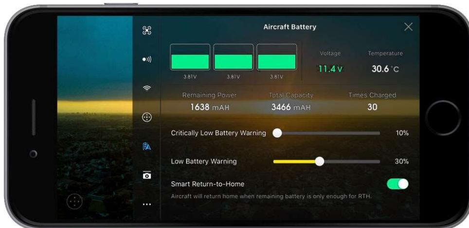
Shows your battery's health. You can adjust Critically Low Battery Warnings and Low Battery Warning percentages here, and this will change when the app sends you a warning about the battery level. Read this article to learn more about your [intelligent battery and how to care for it](#).
